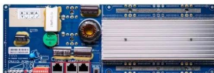
RS485 Communication between battery and inverters Band rate: 9600bps RS485 Interface Communication between parallel packs of BESS and PC Band rate: 9600bps
